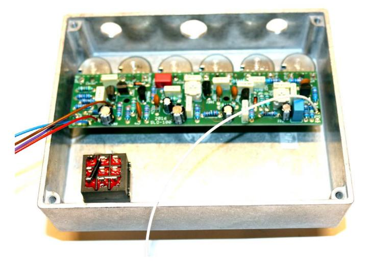
If the board in the enclosure and the Pots tightened nuts, the remaining pins of the potentiometers are firmly soldered.
