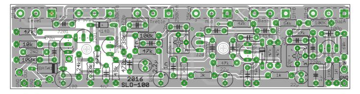
If the board with the components soldered, wires are still in the points GND, Out, +9V, and in LA soldered for the LED. (Soldering point right of the BAT41).
