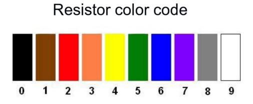
Example: Resistor MF207 10K 1% Value: 10000 Ohm = 10KOhm 1 0 0 2x0 1%
